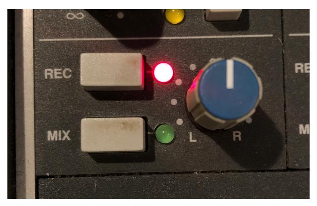
Board mix- assign channel to either Rec or Mix, depending on the monitor source of choice
