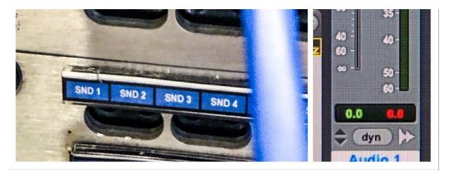
To route to a different channel, plug from Room A Input # to the Mic # of choice, and change the input to the corresponding Input # in Pro Tools
